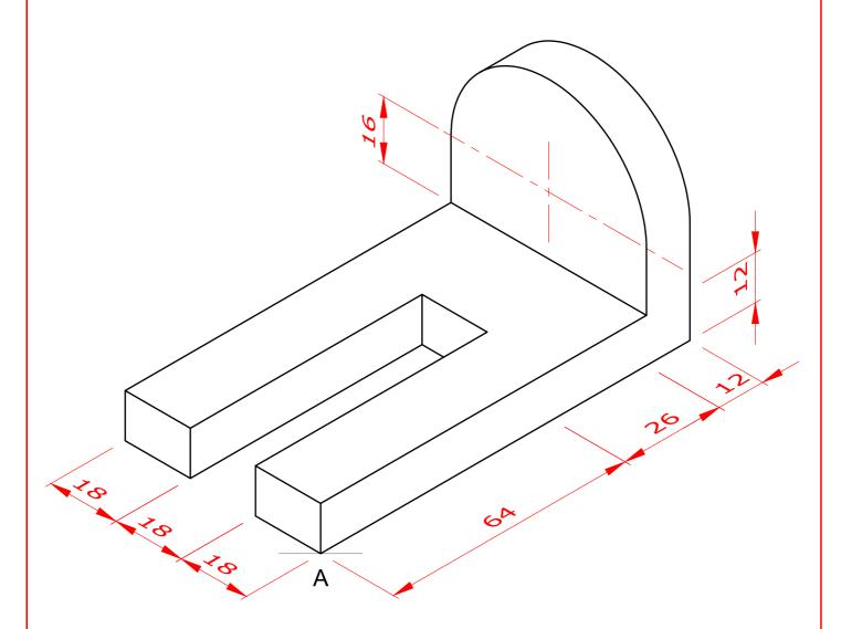
If you have difficulty in drawing this isometric projection, you can use the starter sheet provided to help you. As you improve, try completing the drawing without the use of the starter sheet.
